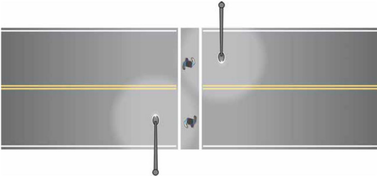
Figure 3-45. Recommended Luminaire Placement at Crosswalk (FHWA, 2008b)
