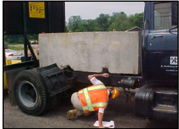
A field technician inspecting a truck mounted attenuator
