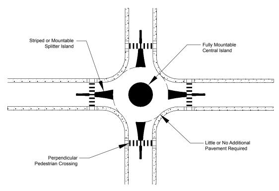
Figure 9-12. Typical Mini-Roundabout
