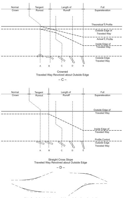
Note: Angular breaks to be appropriately rounded as shown (see text)
