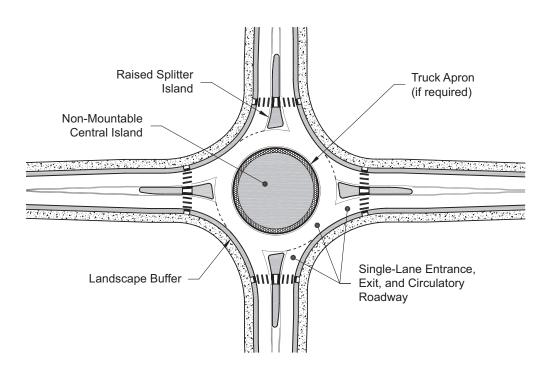
Figure 9-13. Typical Single-Lane Roundabout
