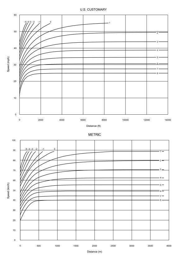
Figure 3-16. Speed–Distance Curves for Acceleration of a Typical Heavy Truck of 140 lb/hp [85 kg/kW] on Upgrades and Downgrades
