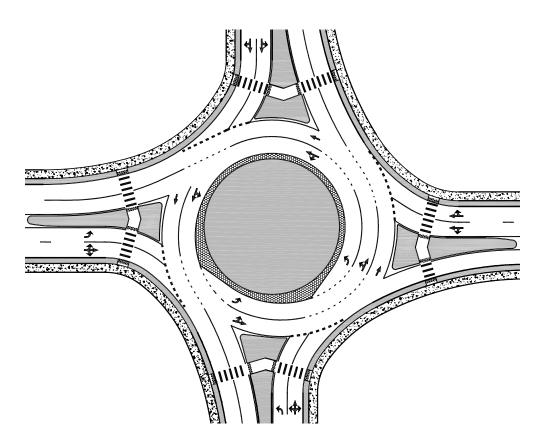
Figure 9-62. Roundabout Lane Configuration Example
