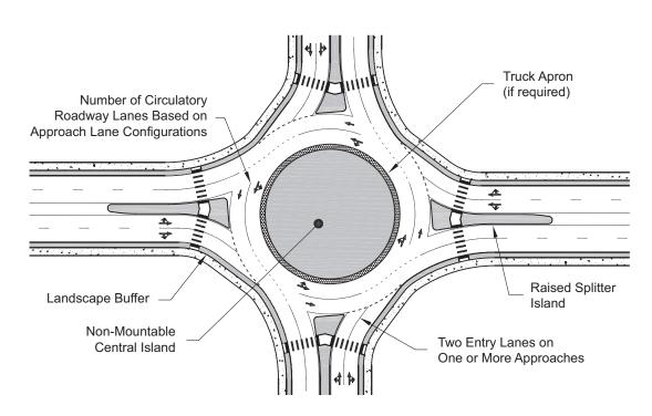
Figure 9-14. Typical Multilane Roundabout
