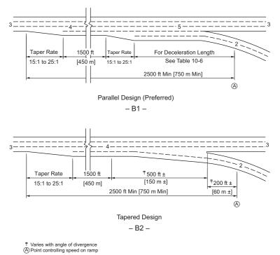
Figure 10-55. Coordination of Lane Balance and Basic Number of Lanes through Application of Auxiliary Lanes
