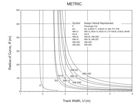
Figure 3-9. Track Width for Widening of Traveled Way on Curves
