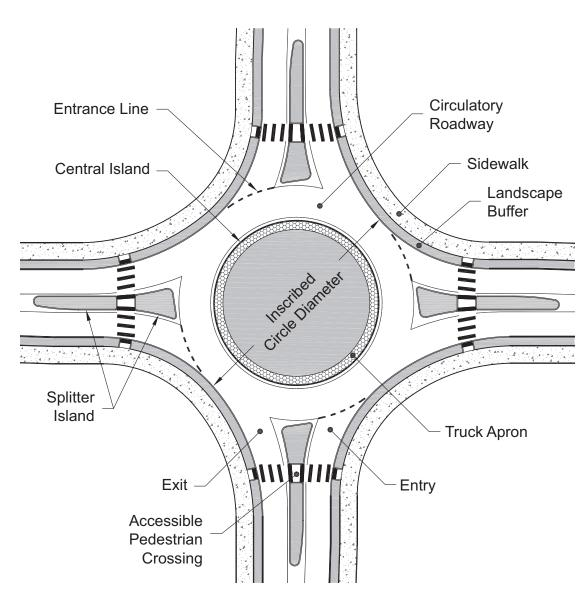
Figure 9-61. Basic Geometric Elements of a Roundabout
